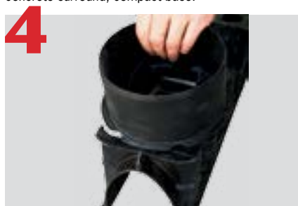
Push-fit outlet adaptor into bottom of channel, lay outlet channel first and connect to 4" or 6" SDR or schedule 40 pipe (Adaptor required for Sch 40).
