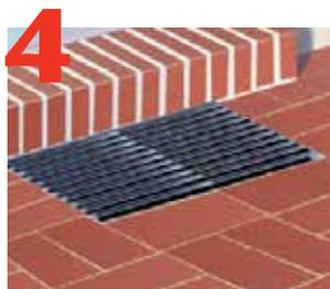
Ensure finished surface is 1/8" higher than the DrainMat to assist water drainage. Fit mat into finished installation.
